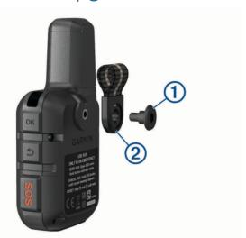
2 Secure the spine mount adapter 1 over the back of the device using the long screw 2 included with the device.
