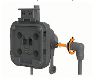
2 Tighten the collar around the connected cable.
