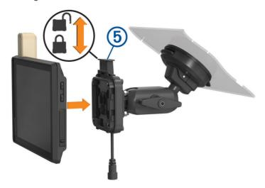
9 Push down the lock (5) to secure the device to the mount.
