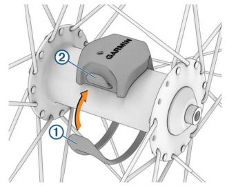
The sensor may be tilted when installed on an asymmetrical hub. This does not affect operation.
