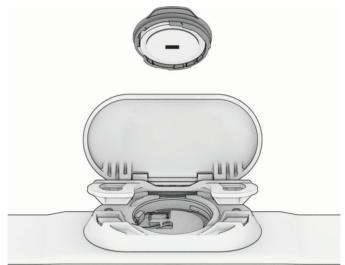
**5** Gently lift the battery out of the cover at the pry point.
