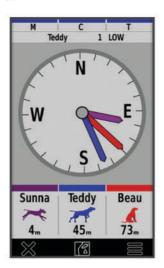
You can use the dog tracking compass to view the direction and distance to your dog, your vehicle, and any paired devices. The dog tracking compass also shows the dog's status, such as running or on point (*Dog Status Icons*, page 12). The color of the pointer corresponds to the color of the track.
